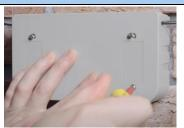
· Fit cover back on and ensure lanyard fits in correctly (doesn't prevent seal of unit).
