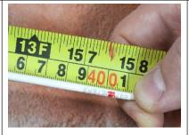
Using a tape measure, mark out the final feeder cable distance measured with tape or reflective pen on the cable.
