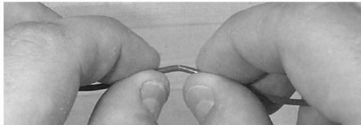
Figure 12 - Flex and separate the tube at the score mark
