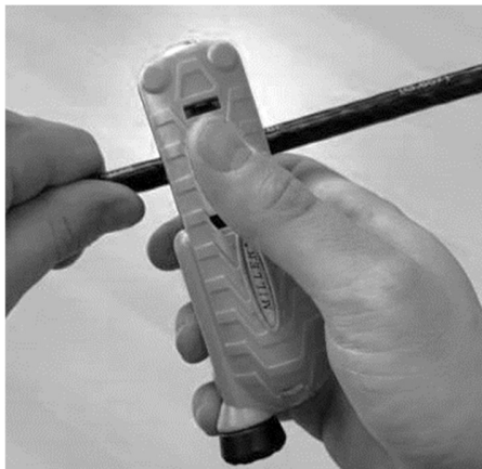
Figure 24 - Ring cut the outer cable sheath
