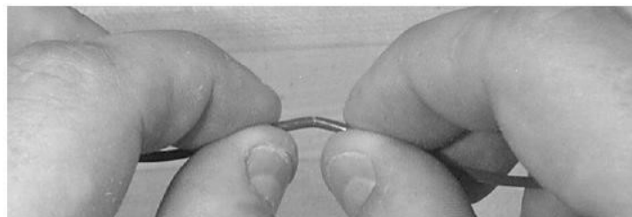
Figure 31 . Separate the buffer tube
