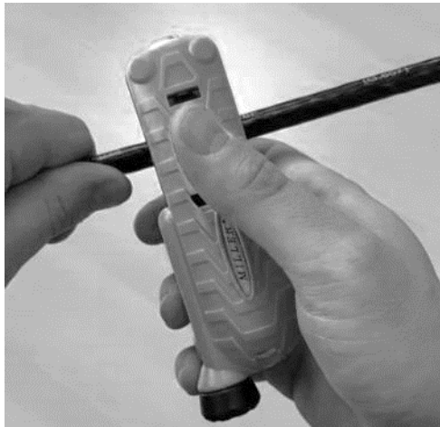
Figure 17 . Ring cut the cable sheath
