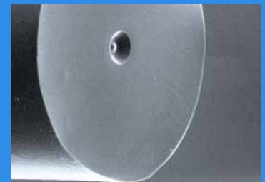
Figure 1. High purity synthetic silica fiber (OFS AllWave ZWP Fiber)
