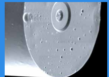
Figure 2. Natural quartz raw material fiber clearly shows many pits and imperfections (competing fiber).
