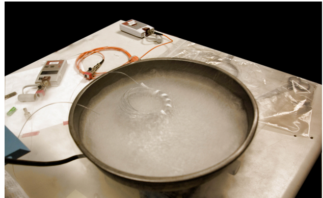
Figure 1: Optical fiber submerged in liquid nitrogen.
